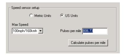
With the radio buttons you can select to use metric (km/h) or US (mph) units. In the left drop-down list you select the max speed to be measured. The SSI-4 measures the speed with a resolution of 0.1 % of the selected max speed.
