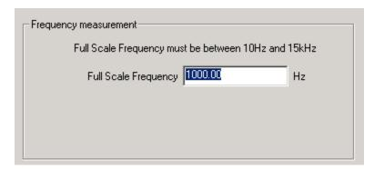
You can enter any frequency between 10 Hz and 15000 Hz as full scale frequency. SSI-4 measures the frequency with a resolution of 0.1 % of the full scale frequency specified. So in LogWorks 0 Hz is always 0 Volt, and the full-scale frequency is equivalent to 5 Volt. This functionality is also available for Inputs 4 and 5.
